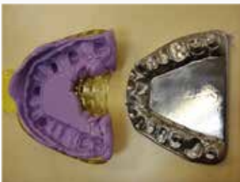
Heavy body (Regular) impression material was poured on the titanium full arch model base for testing
